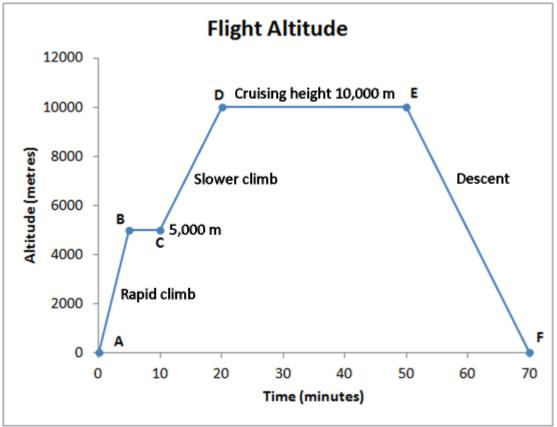
The section from **A** to **B** represents a rapid climb from ground level at Manchester to 5,000 metres in the space of five minutes, followed by a short five-minute spell at that intermediate height from **B** to **C**.
