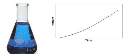
The conical flask narrows towards the neck, and therefore the water level increases at a faster rate as the surface area of the water / air boundary decreases. (We have not included flow into the neck.)
