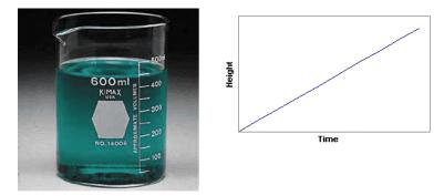
The beaker has constant width, and so the increase in the height of the water follows a straight-line graph. There is no change in the surface area of the water / air boundary.
