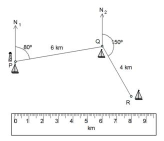
Stage 3: Draw the line PR and measure both its length and the angle it makes clockwise with the northline  $N_1$ .
