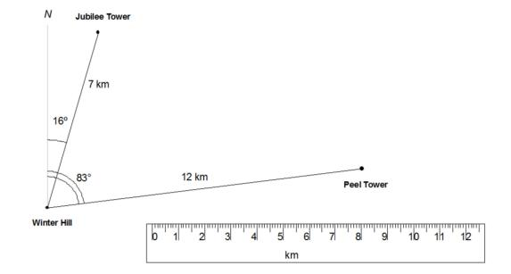
**Stage 3:** Complete the triangle by drawing in the side joining Peel Tower to Jubilee Tower, and draw a northline from Peel Tower. Note how the resulting bearing is a reflex angle, so we measure the smaller acute angle of 63° and subtract from 360° to obtain the true clockwise bearing.
