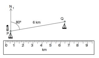
**Stage 2:** Draw another northline  $N_2$  parallel to  $N_1$  at point  $\mathbf{Q}$ . With a protractor centred on point  $\mathbf{Q}$  and the  $0^\circ$  line aligned at northline  $N_2$ , mark a point  $150^\circ$  clockwise from northline  $N_2$ . Complete the line from  $\mathbf{Q}$  passing through the marker point, and plot point  $\mathbf{R}$  4 cm along the line.
