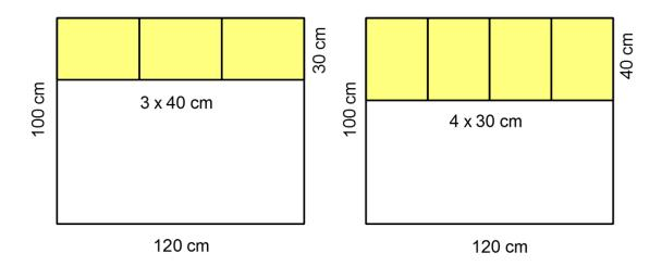
In the first case, we can place three packs to form a row measuring 120 cm by 30 cm; in the second case, the row measures 120 cm by 40 cm.
