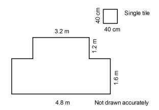
The floor area can be divided up into two rectangles, a larger one of  $(480 \times 160)$  cm and a smaller one of  $(320 \times 120)$  cm. (We have converted metres to centimetres here.)
