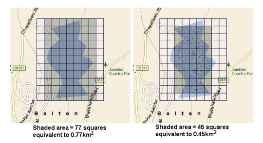
In the diagram on the left, the rectangle has been chosen so that no part of the reservoir is omitted, giving an area of  $0.77~\rm km^2$ . This figure is far too high, because there are many squares containing no part of the reservoir at all.
