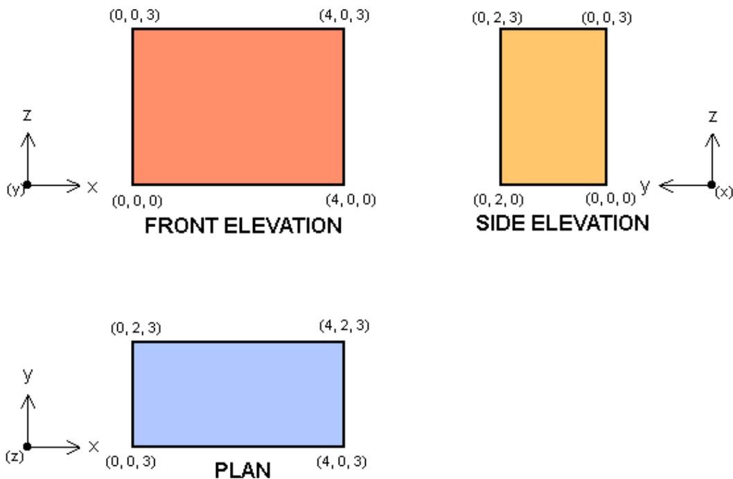
The coordinates of each point have been given here to match with the isometric projection, but again this detail is not needed in exams.
