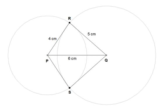
The set of points where **both** conditions are satisfied, i.e. the required locus, is the pair of points where the two circles intersect, shown as R and S in the diagram.
