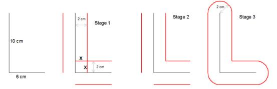
**Stage 1**. Draw two pairs of lines parallel to each of the lines making up the L. Notice that parts of the two lines (inside the corner of the L) are marked with an X. This is because they are 2 cm away from *one* of the line segments, but *less than* 2 cm away from the other, and thus less than 2 cm away from the L-shape as a whole.
